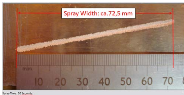
Fig. 5: Erosion crater seen from top with ruler.
